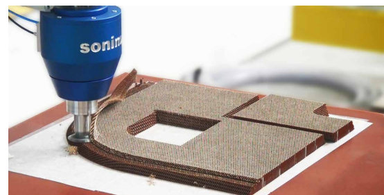
Application on robot cell. NOMEX honeycomb surface machining (thickness 30mm) with Ø63mm disc.
