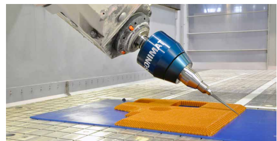
Application on CNC machine : NOMEX honeycomb cutting (thickness 70mm) with 125mm blade.
