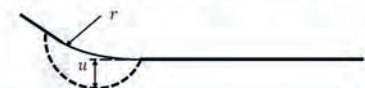
Figure 33 : Surface indention depth after needle peening according to several parameters and surface (DR = Double Radius)
