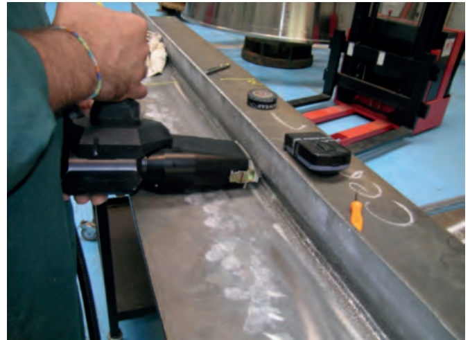
Figure 22: Ultrasonic Needle Peening equipment and operation by SONATS
