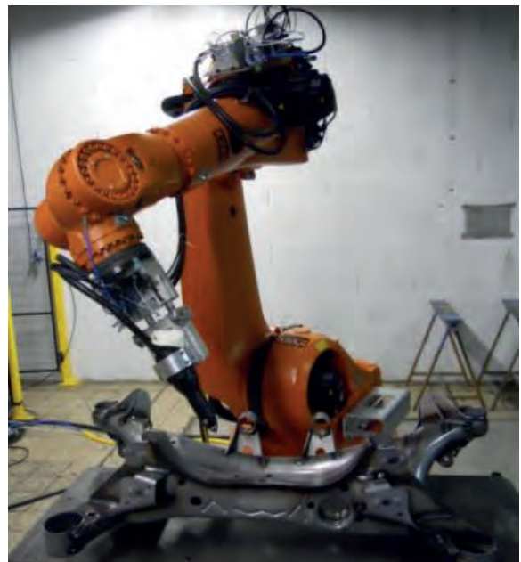
Figure 40 : Robotic UNP on automotive chassis
