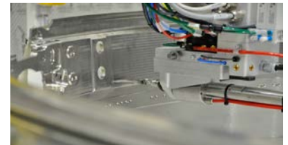
Chamfering after machining of bores and edges
