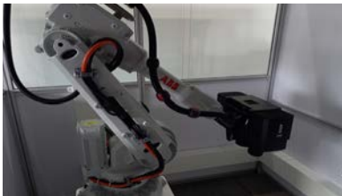
Scanner mounted on robot
